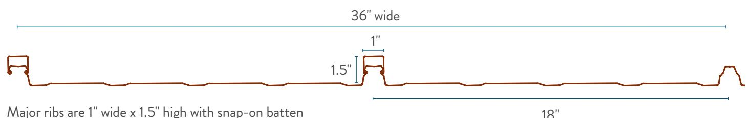
Testing/Approvals: UL 580 Class 90 Wind Uplift, ASTM E 1592 Wind Uplift, UL 2218 Class 4 Impact
